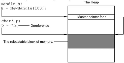
The pointer p now points to the block in memory and we can access the data using it.
