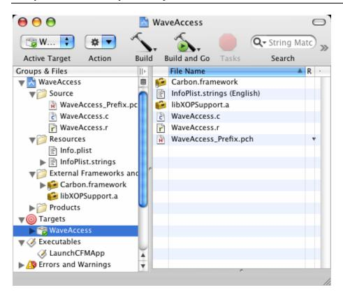
The WaveAccess\_Prefix.pch file is automatically created by Xcode and used to speed up compilation by pre-compiling headers.
