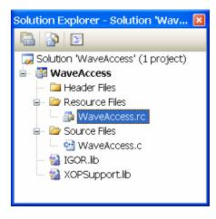
The project is set up to compile either a debug version or a release version of the XOP. You choose which will be built choosing Build-> Configuration Manager. Both of these configurations create an XOP with the same name (e.g., WaveAccess.xop). During development, you will normally compile using the debug configuration. Once your XOP is in final form, you may want to try the release configuration to see if it runs significantly faster.
