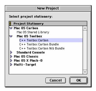
Although we are not using C++, we create a C++ project in case we want to use C++ in the future. The main upshot of choosing C++ here is that the C++ compiler will be used instead of the C compiler and the C++ compiler is more picky about syntax.
