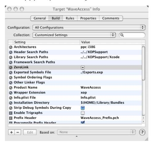
The Architectures controls whether code for PowerPC, Intel or both is generated.
