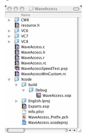
The Xcode project files are inside the Xcode folder, to keep them separate from the files for the other development systems. The discussion assumes this arrangement and we recommend that you use it. Note that the compiled XOP is in the WaveAccess/Xcode/build/Debug folder. Older versions of Xcode used the term Development instead of Debug.
