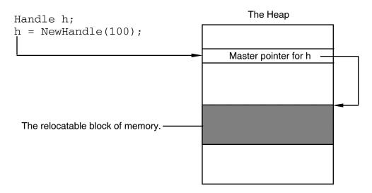
A block allocated by NewPtr is called non-relocatable. A block allocated by NewHandle is called relocatable. Using handles allows the memory management system to avoid heap fragmentation by moving relocatable blocks when it needs to allocate a new block.
