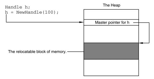
The benefit of this is that the memory manager can move the block to make room for other blocks. The memory manager updates the master pointer so that it points to the new location of the block. The handle still points to the master pointer and thus is still a valid reference to the block.
