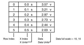
For a 1D wave, the row indices are also called point numbers. The X indices are calculated by Igor from the row indices using the scaling information for dimension 0 of the wave. You can set this scaling using a "SetScale x" command from within Igor and using the MDSetWaveScaling XOPSupport routine from an XOP. You can set the X units using a "SetScale x" command from within Igor and using the MDSetWaveUnits operation XOPSupport routine from an XOP.
