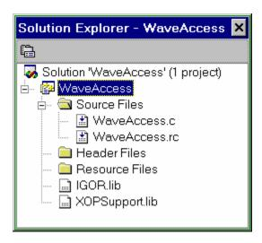
The project is set up to compile either a debug version or a release version of the XOP. You choose which will be built choosing Build-> Configuration Manager. Both of these configurations create an XOP with the same name (e.g., WaveAccess.xop). During development, you will normally compile using the debug configuration. Once your XOP is in final form, you may want to try the release configuration to see if it runs significantly faster.
